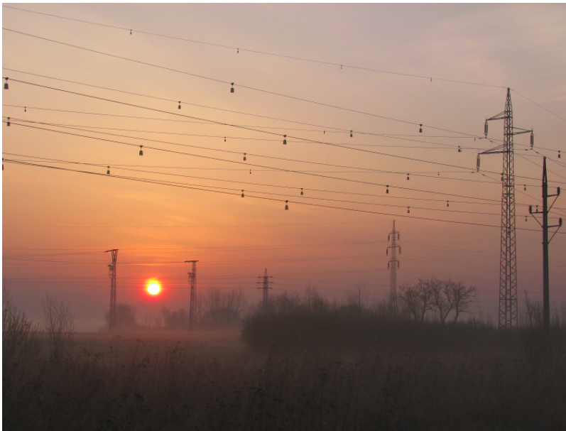
Figure D.4: FireFly Bird Diverters are able emit luminescent light at twilight and at night.
