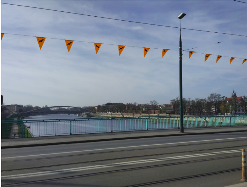
Figure D.7: Flags to prevent bird collisions attached on trolley wires in Krakow. Source: Raptor Protection of Slovakia
